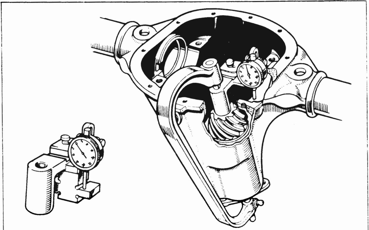
Fig. D.7 CHECKING PINION SETTING DISTANCE
