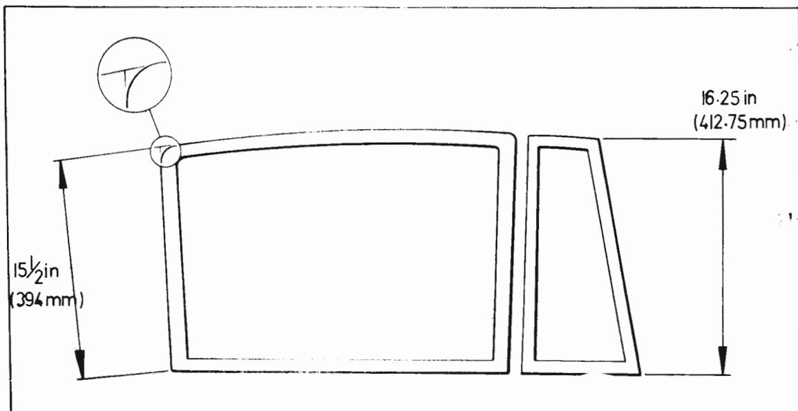
Fig. P18. Setting dimension for door drop glass and quarter lights.
