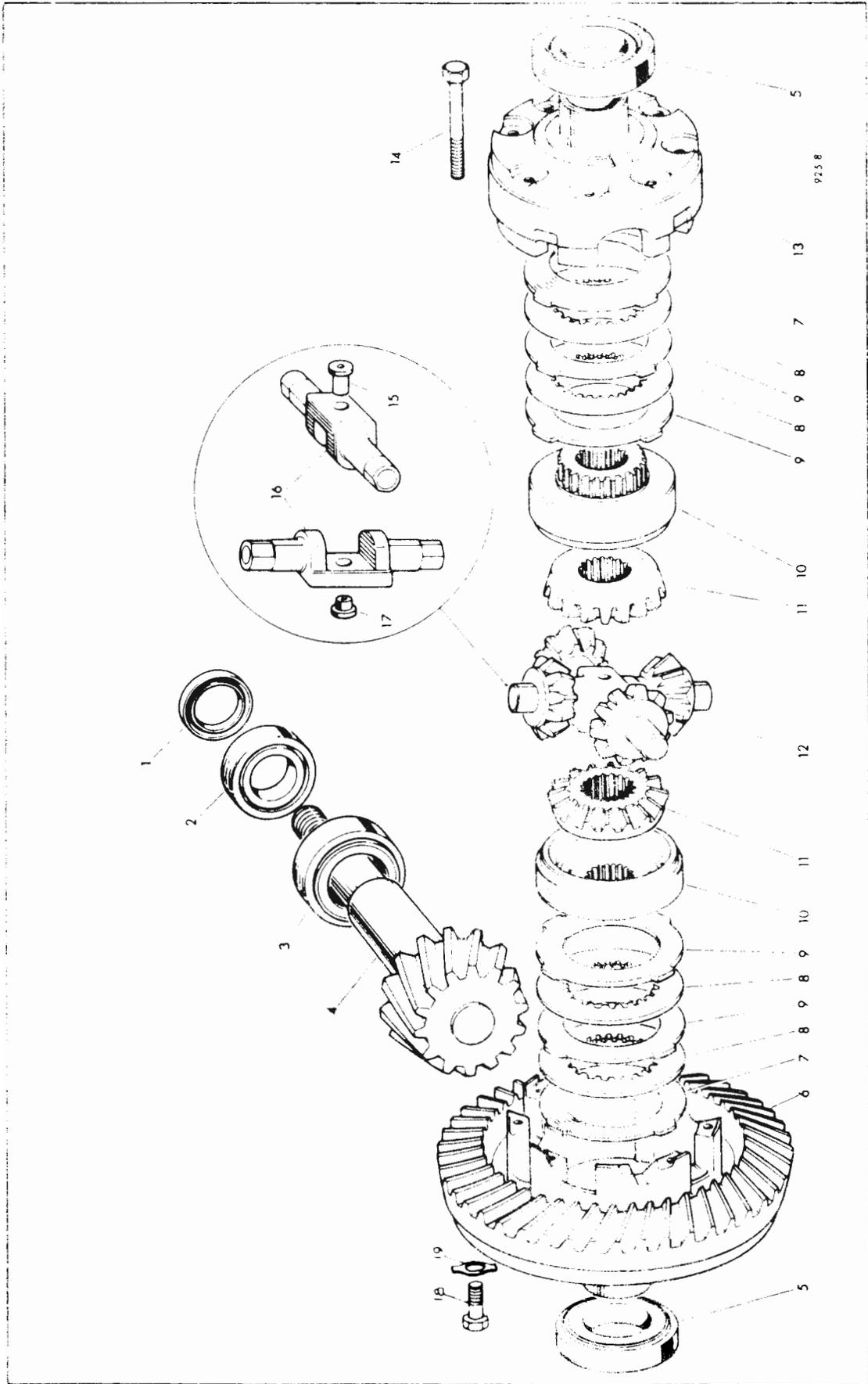
Fig. 6.3 'POWER-LOK' DIFFERENTIAL & DRIVE GEARS
