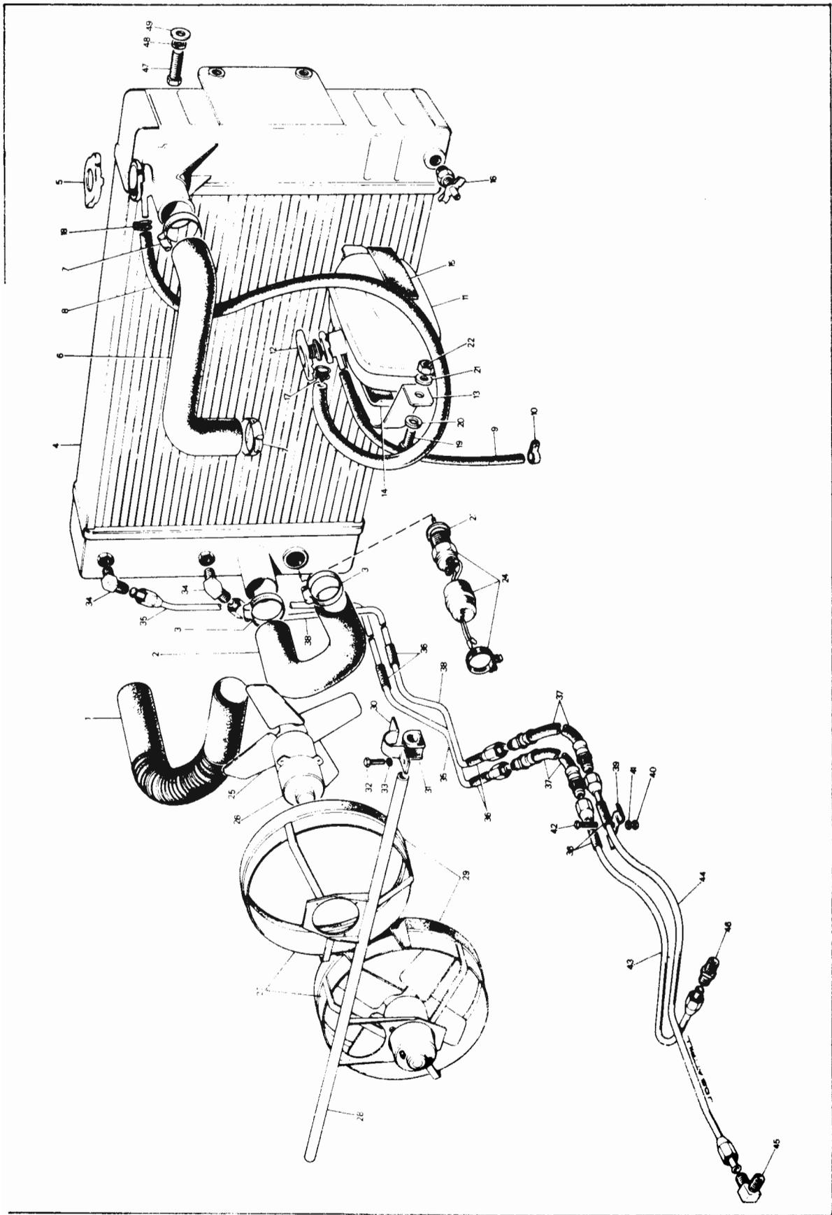
Fig. L.4 Radiator and Cooling System
