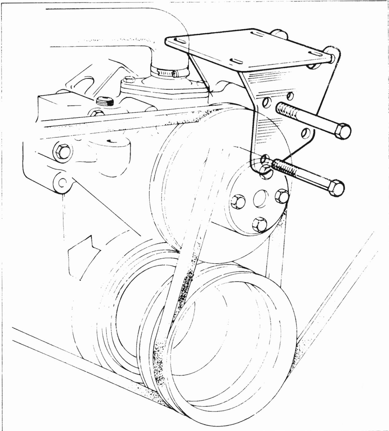
Fig. MA.5 Details of Compressor Mounting bracket and bolts
