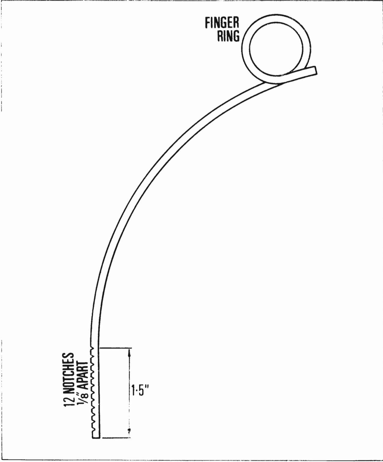
Fig. MA.4 Compressor Dipstick Details
