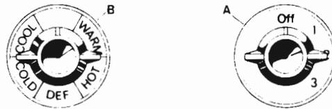
As the master switch (A) controls not only the electrical circuits but also the vacuum system operating the flap valve on the air intake, it is essential that this switch is operated before the heater will function. In addition to the heater OFF position, the three positions provide for RAM air, and slow or fast fan operation.
