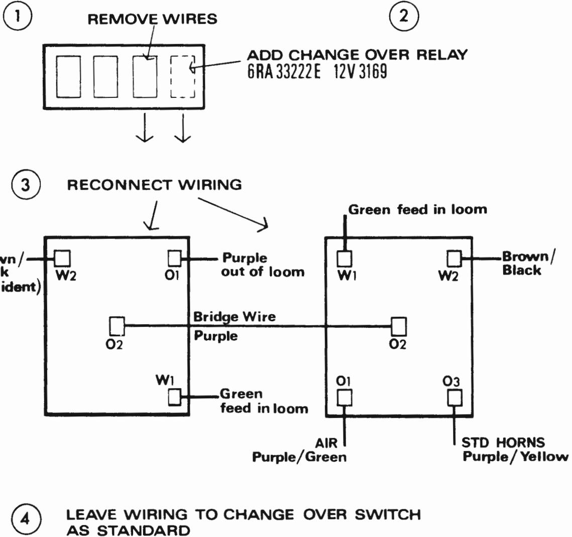
Fig. N.6 Wiring changes for fitting air-horns on Mk.11 cars
