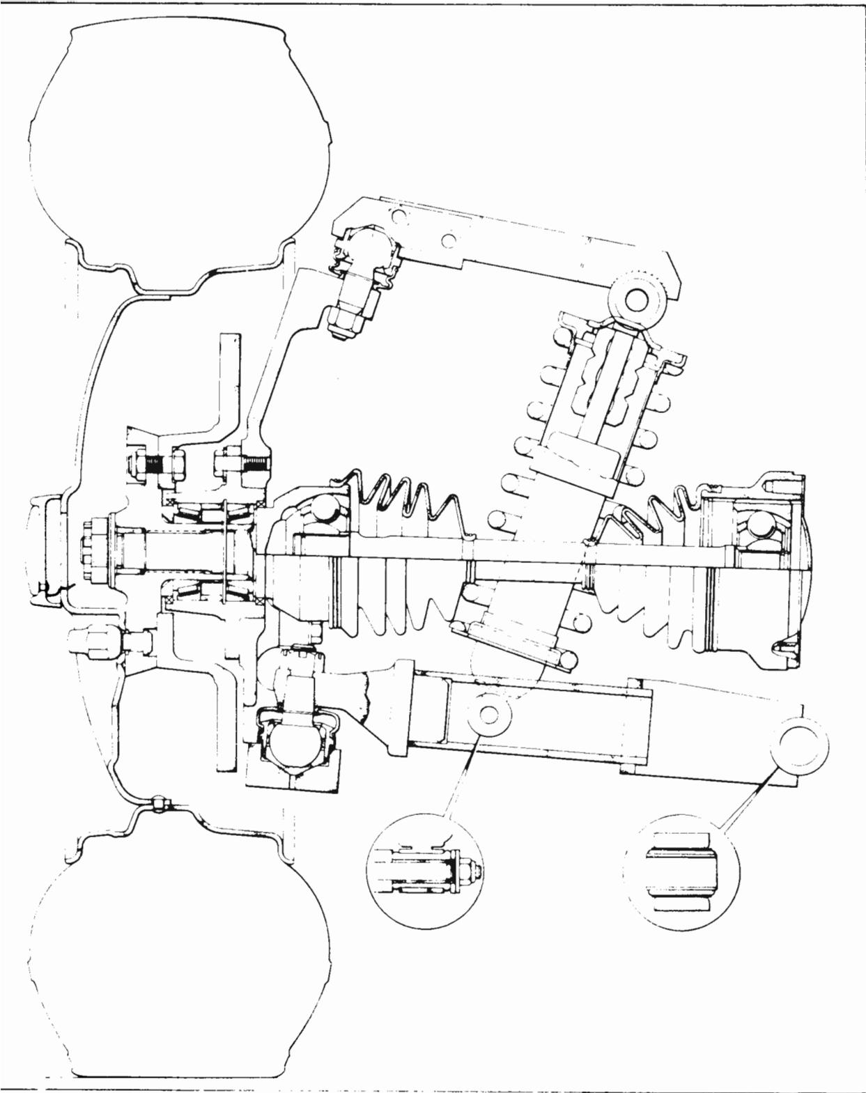
Fig. C.11 FRONT SUSPENSION - CROSS SECTION
