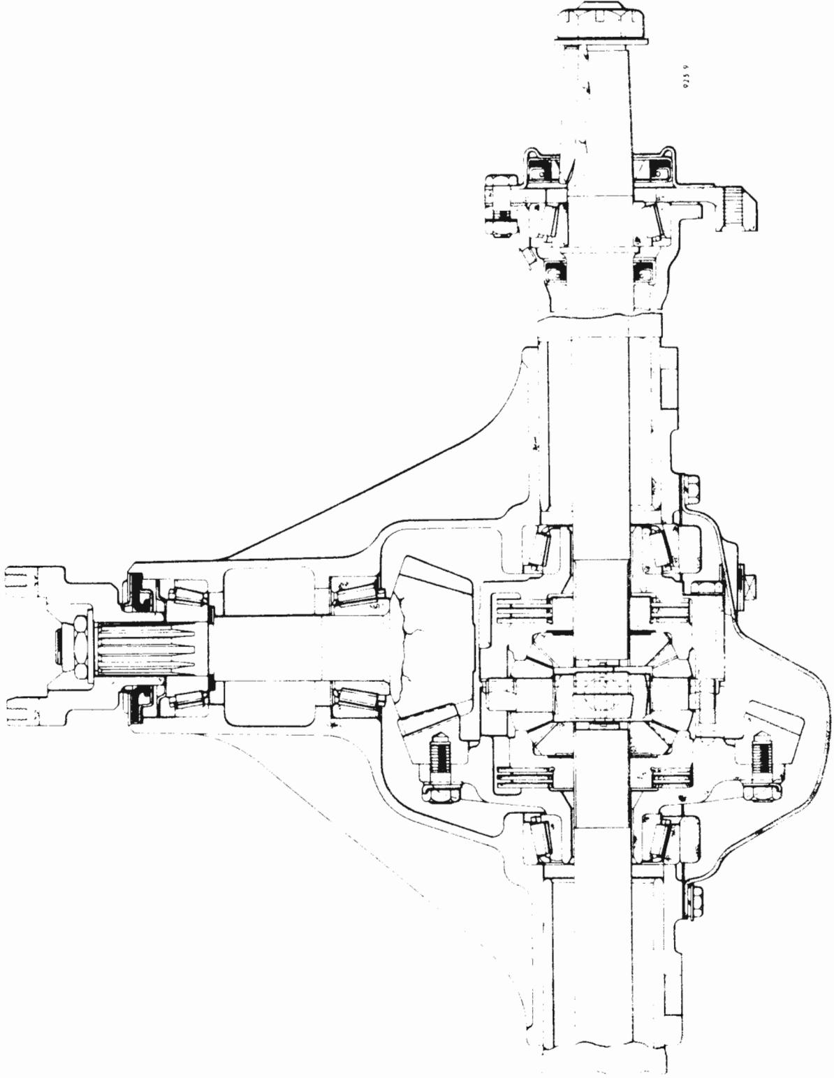
FIG. D.2 CROSS-SECTION OF REAR AXLE
