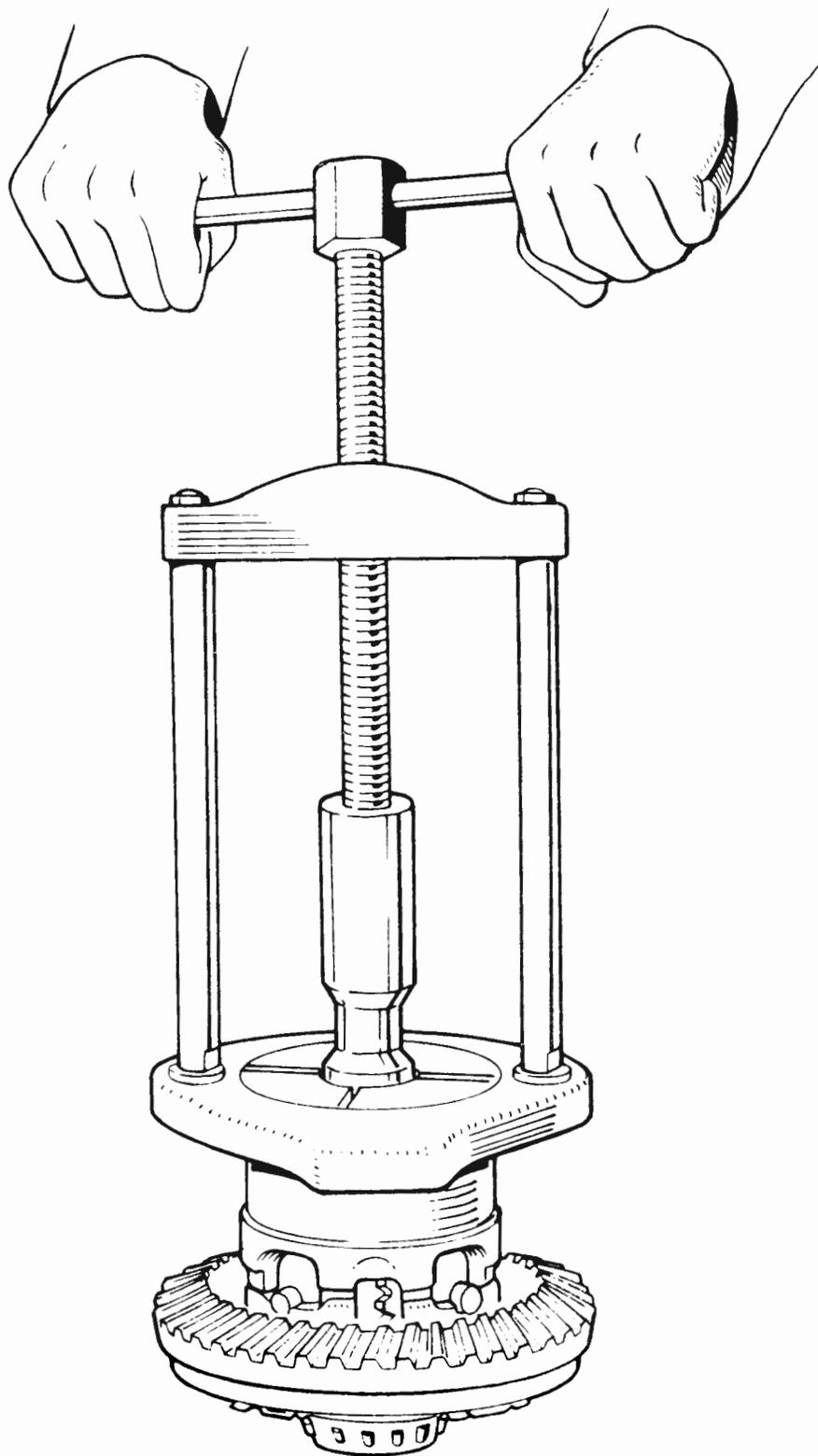
Fig. D.4 WITHDRAWING A DIFFERENTIAL BEARING USING TOOL NO. SE.103
