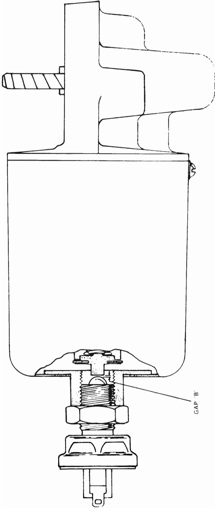
SET GAP B TO 0.005 in BY SCREWING IN SWITCH UNTIL ELECTRICAL CONTACT IS MADE AND THEN UNSCREWING **EXACTLY** HALF A TURN
