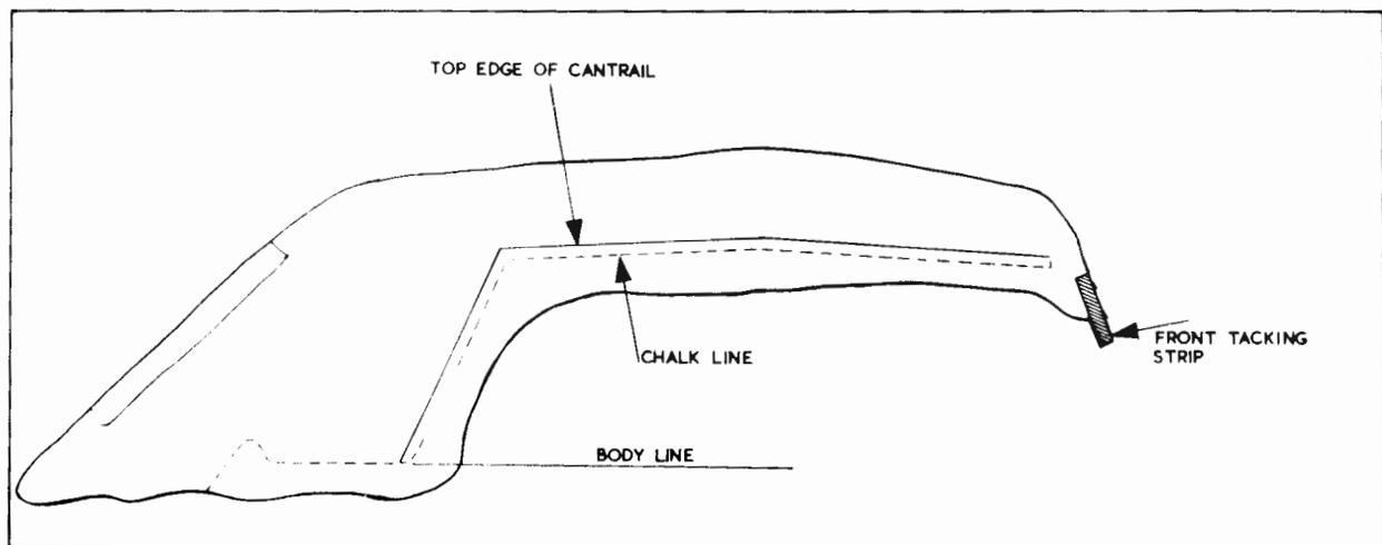
Fig. P4B - Marking roof outer fabric
