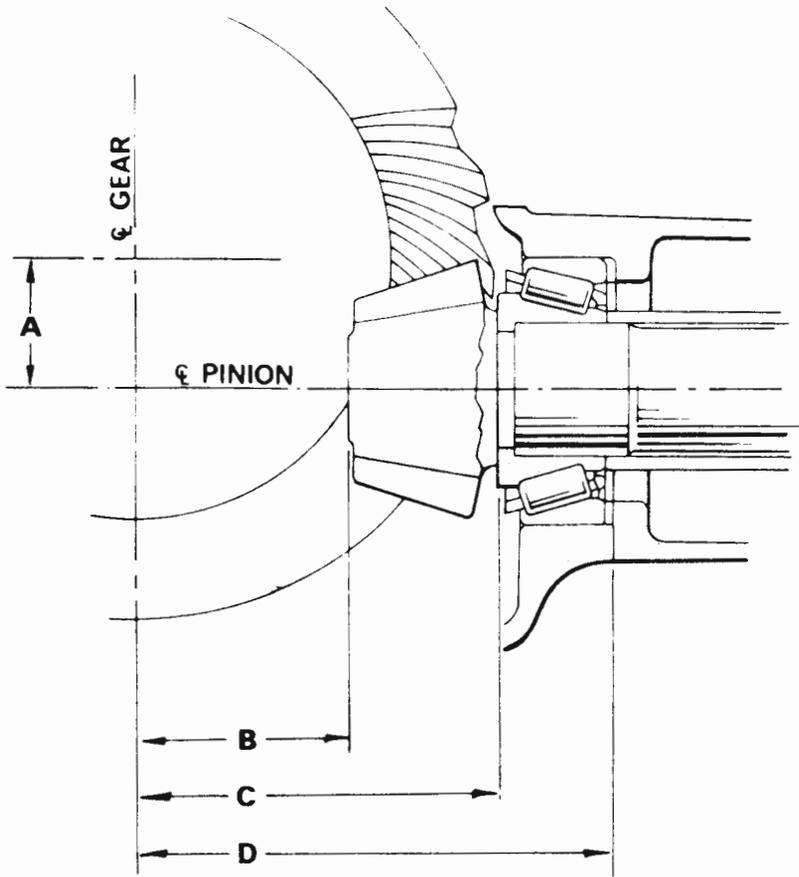
Fig. D.6 PINION SETTING DISTANCES
