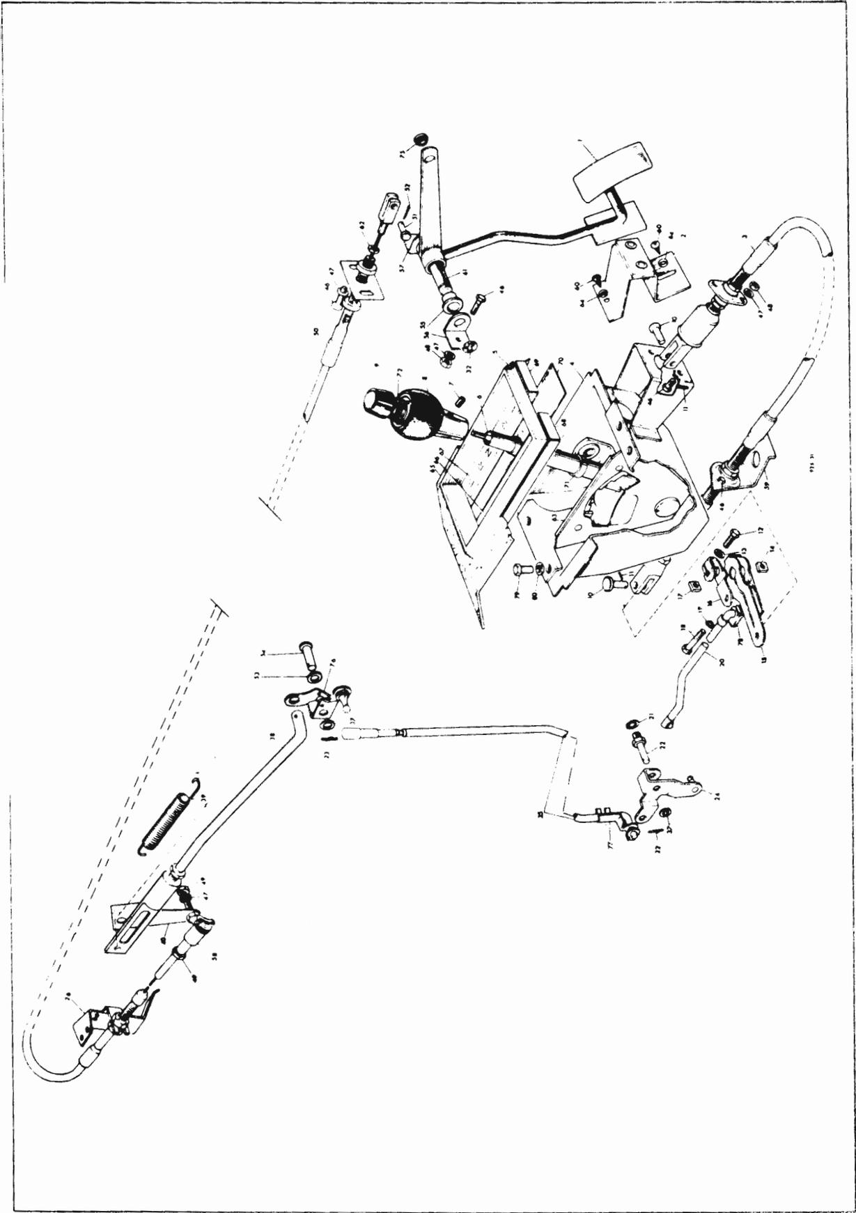
Fig. K.4 Accelerator and Gear Shift Control
