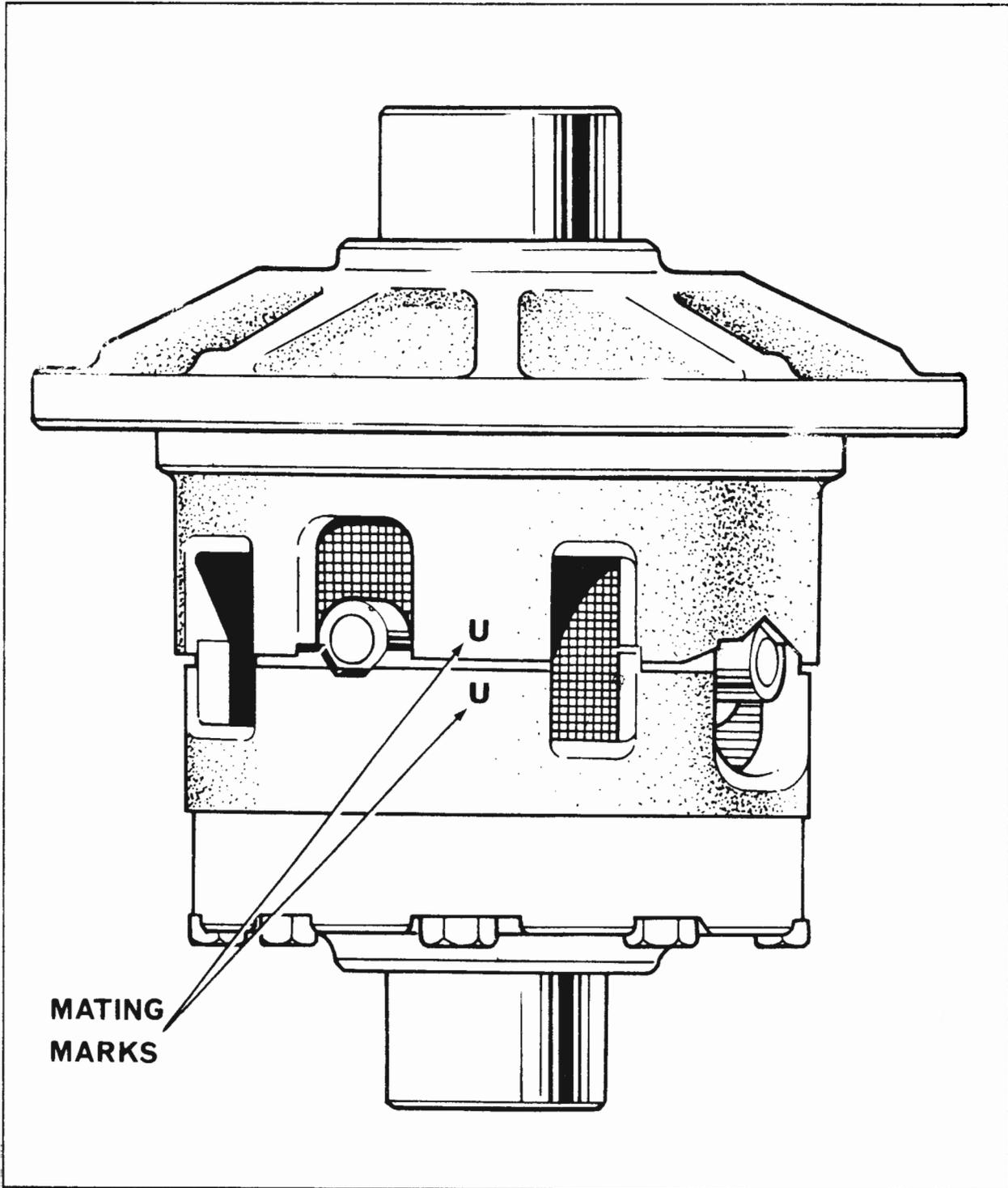
Fig. D.5 ALIGNMENT MARKS ON DIFFERENTIAL CASING
