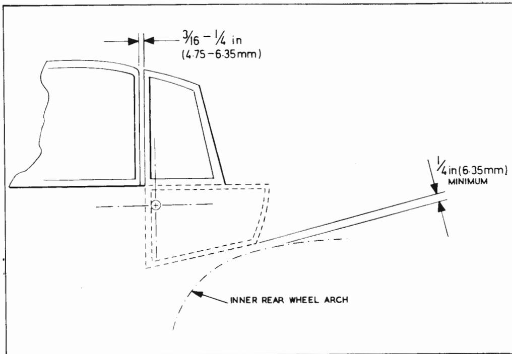
FIG. N13B. ADJUSTMENT OF REAR QUARTER LIGHTS
