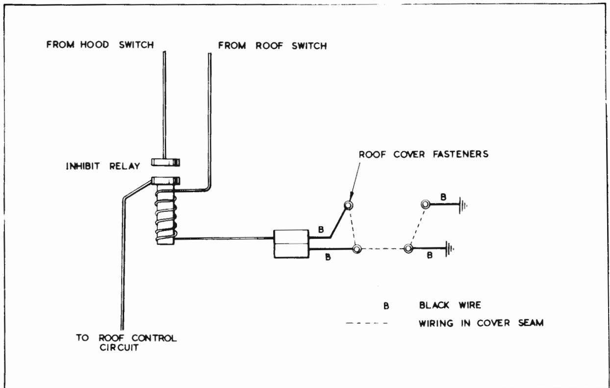
FIG. N11B. ROOF COVER INHIBIT RELAY
